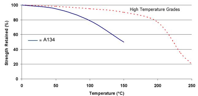
The reduction in strength shown here is reversed on cooling providing the joint is not overstressed. Exposure to higher temperatures may be acceptable for short periods
