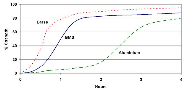
Cure times are typical at 23°C. Copper and its alloys will follow the faster cure while oxidised or passivated surfaces like stainless steel will tend towards the slower curve. Lower temperatures or large gaps will tend to extend the cure time. To reduce the cure time the use of Permabond A905, or heat, can be considered.
