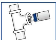
For taper/parallel threads ensure adhesive is positioned where the threads will engage fully. Gaps, and therefore cure times, may be greater than expected with this joint configuration.
